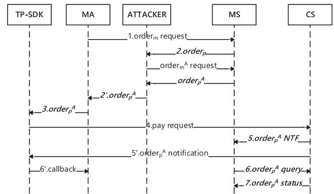
Fig. 6. Order Substituting Attack to process model II.
