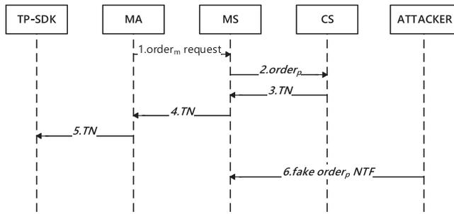
Fig. 5. Notification Forgging Attack to process model I.
