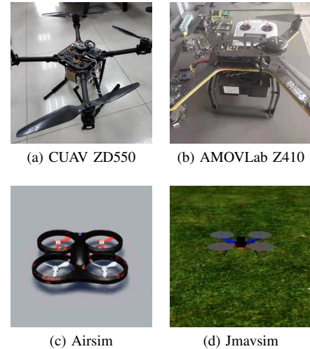
Fig. 3: Real and virtual drone vehicles used for experiments.
