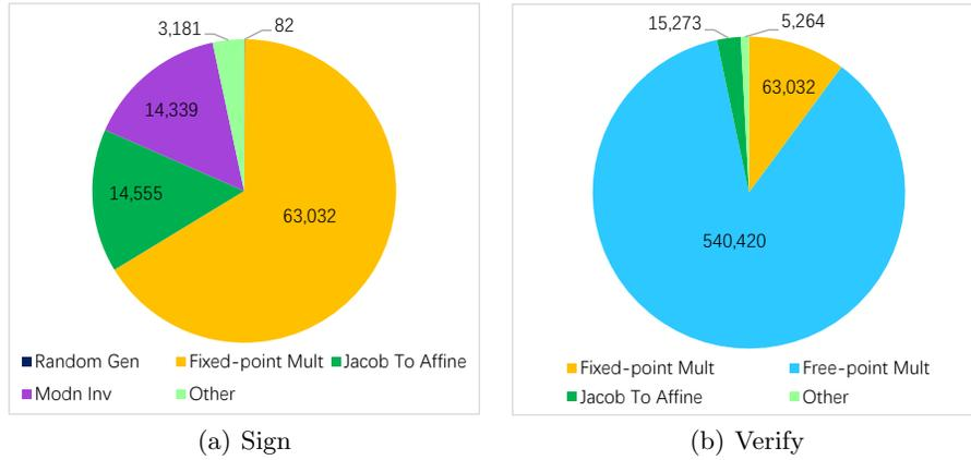
Fig. 4. Instruction consumption of each module in Yog-SM2
