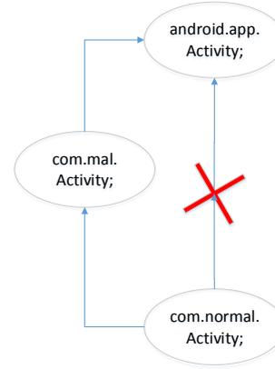
Figure 2: Entry Point Class Inheritance Modification
